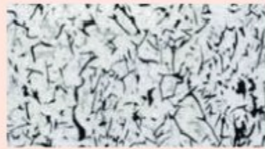
Flaky Graphite in Grey Cast Iron
