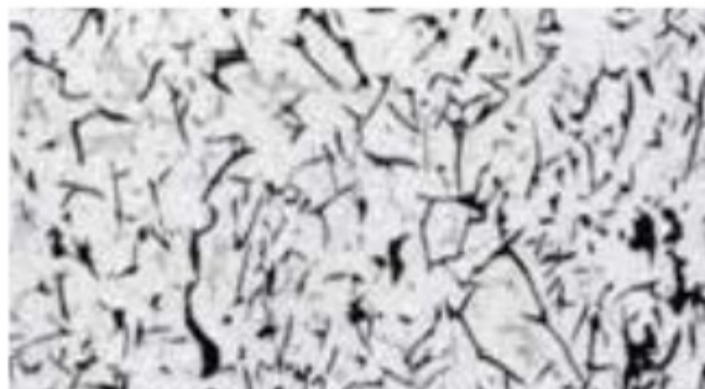
Flaky Graphite in Grey Cast Iron
